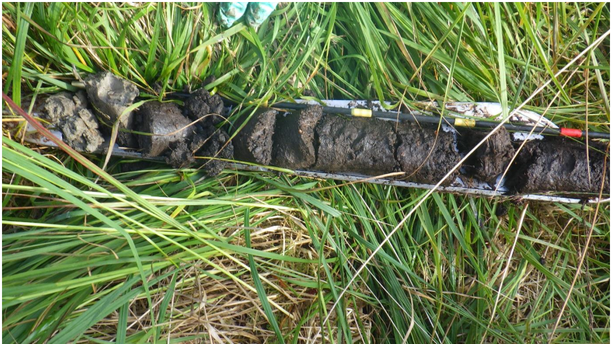
Notes: View showing interior of core sections. Primarily moderately decomposed peaty soils overlying clay at base (left of photo)
